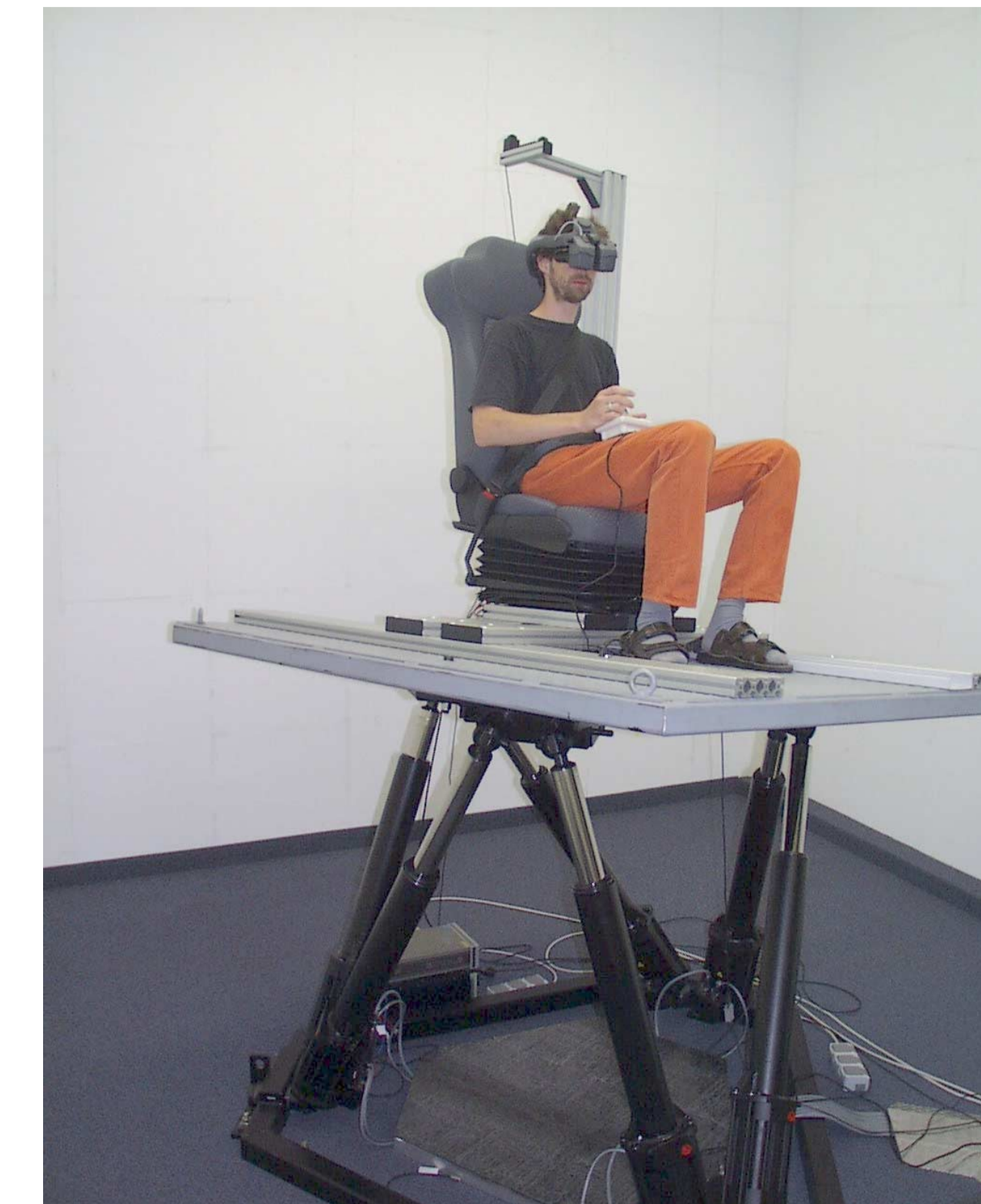
Figure 3: Motion platform with six degrees of freedom for the vestibular stimulus.
