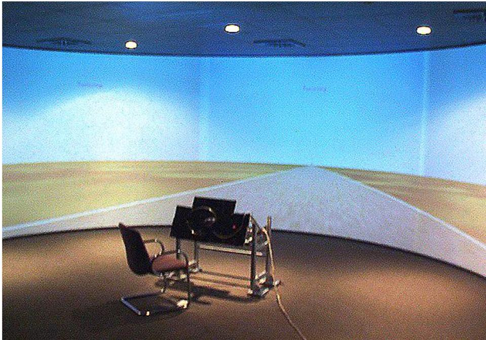
**Figure 1.** The experimental apparatus and virtual reality environment used in these experiments. Shown here is the projection screen at the start of a trial. The simulation began with the car in the center of the street, but always had a small, random deviation in the heading direction of the car, forcing the subject to engage in minor corrective steering behaviors from the beginning of each trial. The projection screen was a half-cylinder with a diameter of 7.5 m and a height of 3.15 m.
