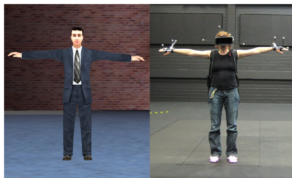
Figure 1: The self-avatar (left) is used to represent the participant's body (right) within the VE. The body movements of the participant are directly linked to the movements of the self-avatar using inverse kinematics.
