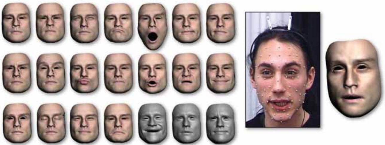
Figure 1: An Action Unit basis obtained from 3D scans and texture (left) and a Motion Capture system. Expressions can be retargetted frame-by-frame from Motion Capture to morph shapes by automatic decoding and application of Action Unit activation levels (right).
