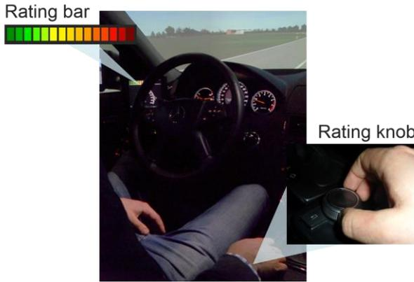
Figure 4. Location of rating bar and rating knob in car cabin.
