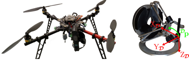
Fig. 1: Left: the quadrotor setup at date (i.e., without the Odroid board). Right: the haptic device and its frame of reference.
