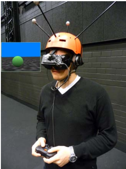
Fig. 2. Participant wearing a HMD; his view (target sphere above textured ground plane) is indicated in the inset.
