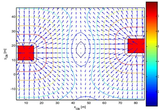
Fig. 2. Sample obstacles-generated force field.
