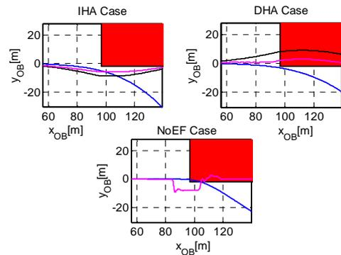
Fig. 7. Isolated obstacle scenario: IHA, DHA and NoEF experiments in the Maximum Fog visibility condition. The obstacle is drawn in red. The lines represent: the aircraft trajectory (blue) starting from the left, the force  $F_E$  (magenta when present) and the total force  $F_{S,yOD}$  (black).
