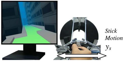
Fig. 1. The experimental setup. Upper left section shows a sample out of the window view of the scenario; lower right shows the Omega Device and the Y axis degree of freedom.
