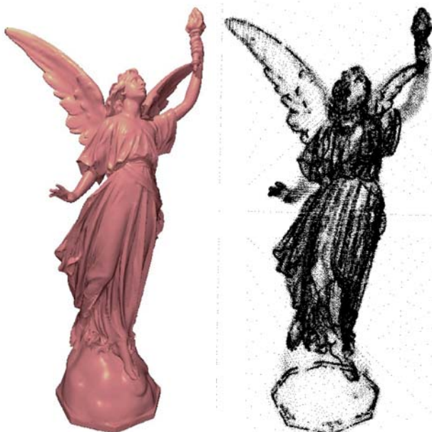
1(a). Rendered implicit surface model of “Lucy”, constructed from 56 million data points. (b) The center locations of the 364,982 compactly supported basis functions which are used to define the surface.
